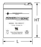
L: 3.86 (98) W: 4.40 (112) H: 4.65 (118) HT: 4.65 (118) Tolerances are +/- 0.04 in. (+/- 1mm) and +/- 0.08 in. (+/- 2mm) for height dimensions. All data subject to change without notice.
